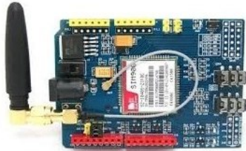
Fig 3. Shield GSM/GPRS SIM 900
